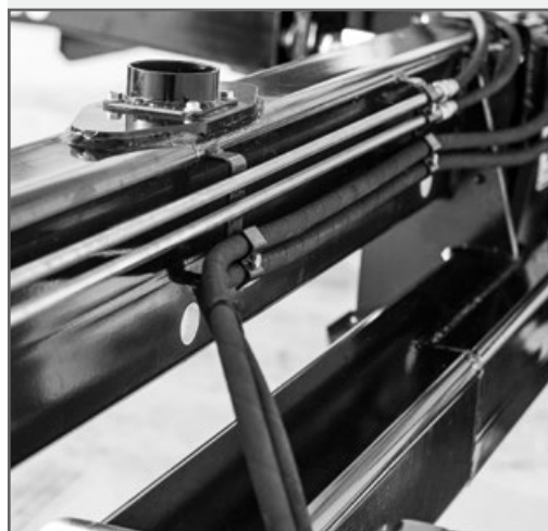
INTRA-AIRWAY™ vacuum port located inside 9x5 tube Keeps bar free of extra lines & clean for maintenance & service
