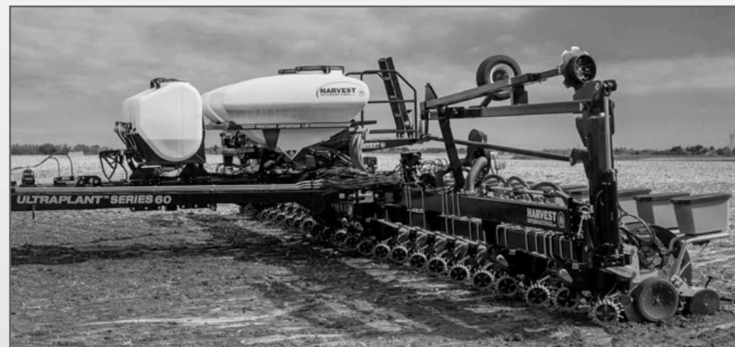
60' UltraPlant & LaserPro1 units 24 row 30" spacing; CSD, 500 gal liquid, vDrive insecticide mount UltraPlant Model: PB6030BR
